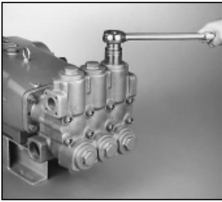
Removing Valve Plug (6760)
