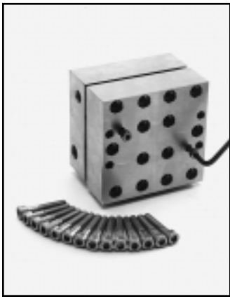
781 Removal of Valve Block Manifold
